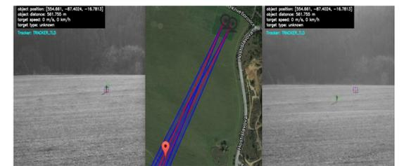
As for the static targets, nine landmarks with a priori known UTM coordinates (obtained from the cadastral map) and one target carrying an ordinary mobile GPS sensor were chosen. The system was tested against one dynamic terrestrial target equipped with a mobile GPS sensor (a walking person) as well. The target was tracked for 120 s and the estimated positions were captured and compared to the ground truth path; on average the system achieved the precision of 6.25 m.
