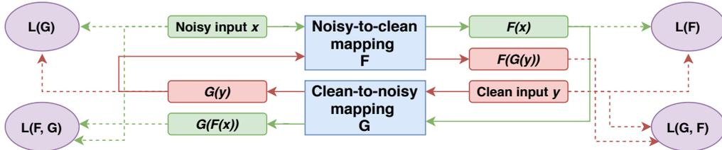
**Figure 3.** The architecture of cycle-consistency training framework for speech enhancement (CSE). Based on [7].
