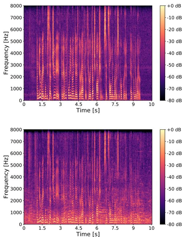
**Figure 1.** Comparison of clean and corrupted speech signal spectrogram.
