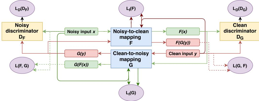
**Figure 4.** The architecture of adversarial training framework with cycle-consistency for speech enhancement (ACSE). Based on [7].
