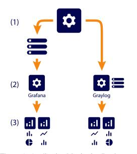
**Figure 8.** Application Monitoring Deployment This figure shows the current monitoring deployment. (1) The application produces data into the database (left branch) and logging messages (right branch). (2) The monitoring systems process the data independently. (3) Data are aggregated and presented understandably.
