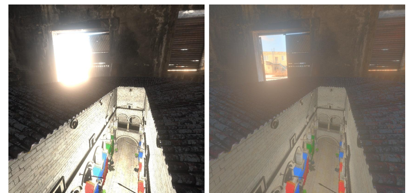
Figure 5: Results of Bilateral Filter local tone mapping. HDR input (left) vs. tone-mapped (right).
