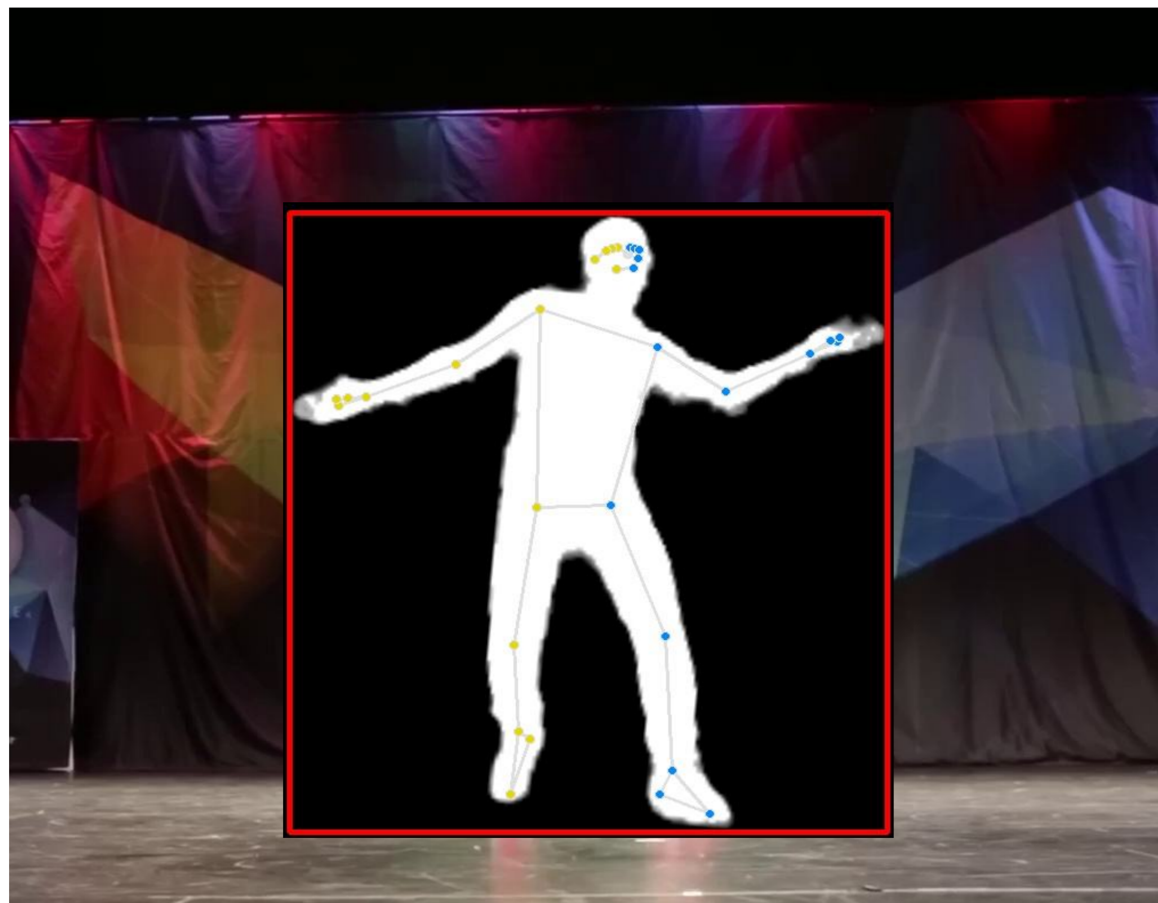
Figure 1: MediaPipe Pose segmentation mask or YOLO detector are used to calculate the bounding box around the person's body. Body landmarks are used in body parts crop (Figure 5).
