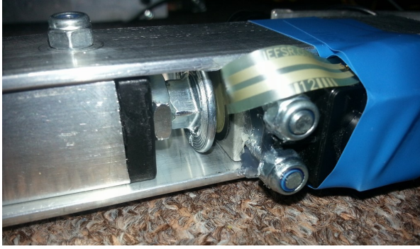
Figure 3. Force-sensitive resistors placement. The inner profile is movable in digits of singles a millimeter. This ensures perfect functionality of the force-sensitive resistor.
