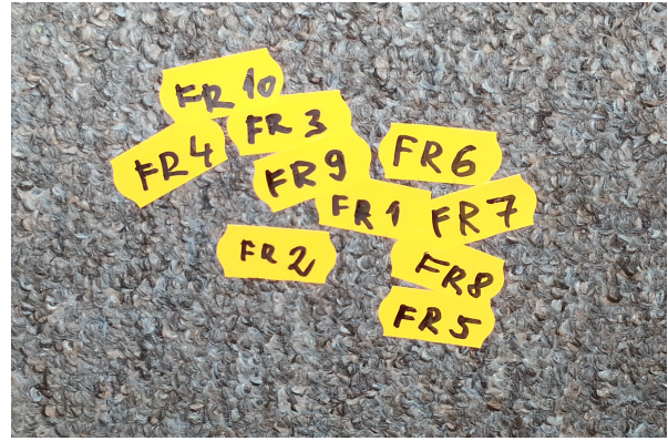
Figure 7. Results of repeatability of movement. This figure shows the results of all attempts during the testing of the repeatability of the robot movement. Each sticker represents one final position of a footer. The number on the sticker is an attempt number.
