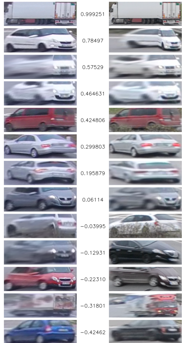
Figure 10. Results (numbers in the middle) of deep regressions (several random regressions per one vehicle pair) from 10,000 randomly generated vehicle pairs. The more similar the vehicles are, the higher regression result is computed. From the experiment it can be assumed that almost all positive regression results belong to similar-looking vehicle pairs.
