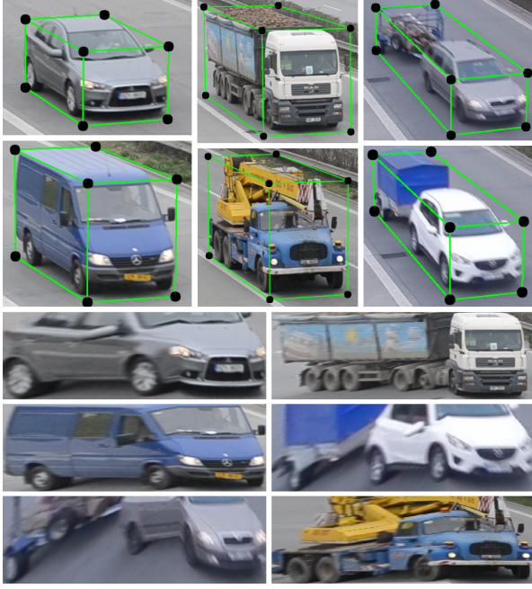
Figure 1. Examples of detections. Data received from the detection system are represented as seven points describing the 3D bounding box around the detected vehicle. Under the detection examples are results of image extraction from the 3D bounding box.
