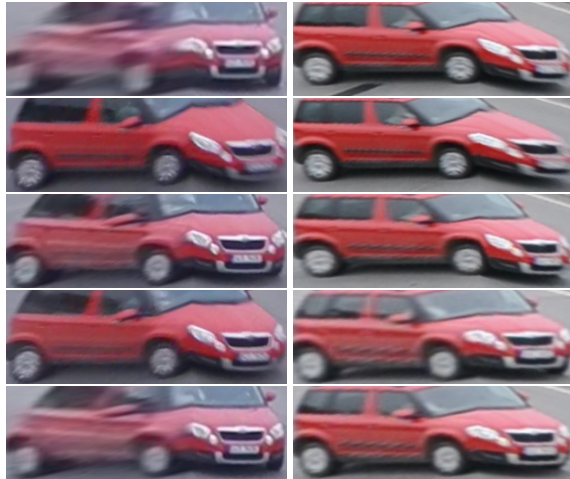
Figure 9. Randomly generated positive pairs of the same vehicle for the linear classifier training. left: Camera A, right: Camera B.
