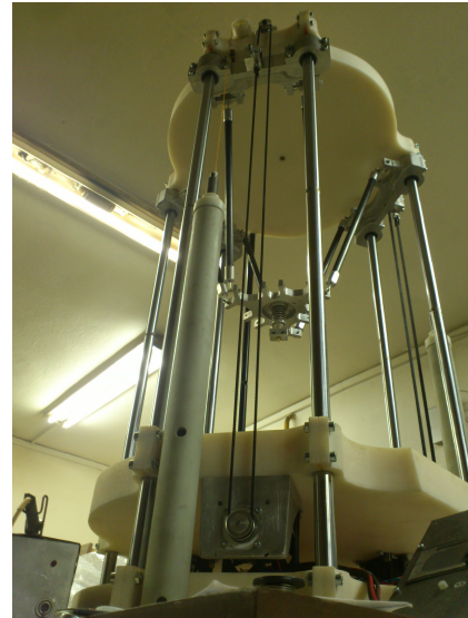
Figure 6. The principle of the counterweights' utilization.
