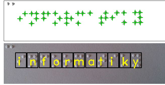
Figure 4. The top image shows a final line of correctly detected dots. Distances between dots are measured, and the dots are grouped into particular characters. The final output of the process is shown in the bottom image. The characters are correctly detected, translated and rendered back on the screen.
