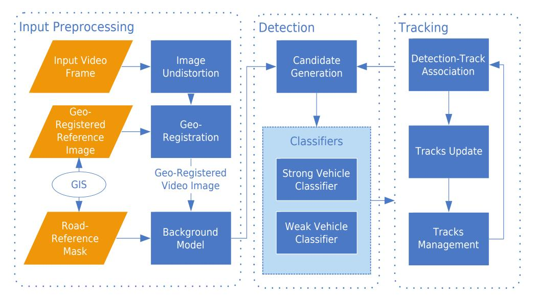
The detection candidates are analyzed by two vehicle classifiers - strong vehicle classifier which produces confident detection cues, and weak vehicle classifier which provides tracking attractors to aid multi-target tracking. The classifiers use Multi-Block Local Binary Pattern features and are constructed by AdaBoost algorithm on dataset of 20,000 hand annotated vehicles and road structures.
