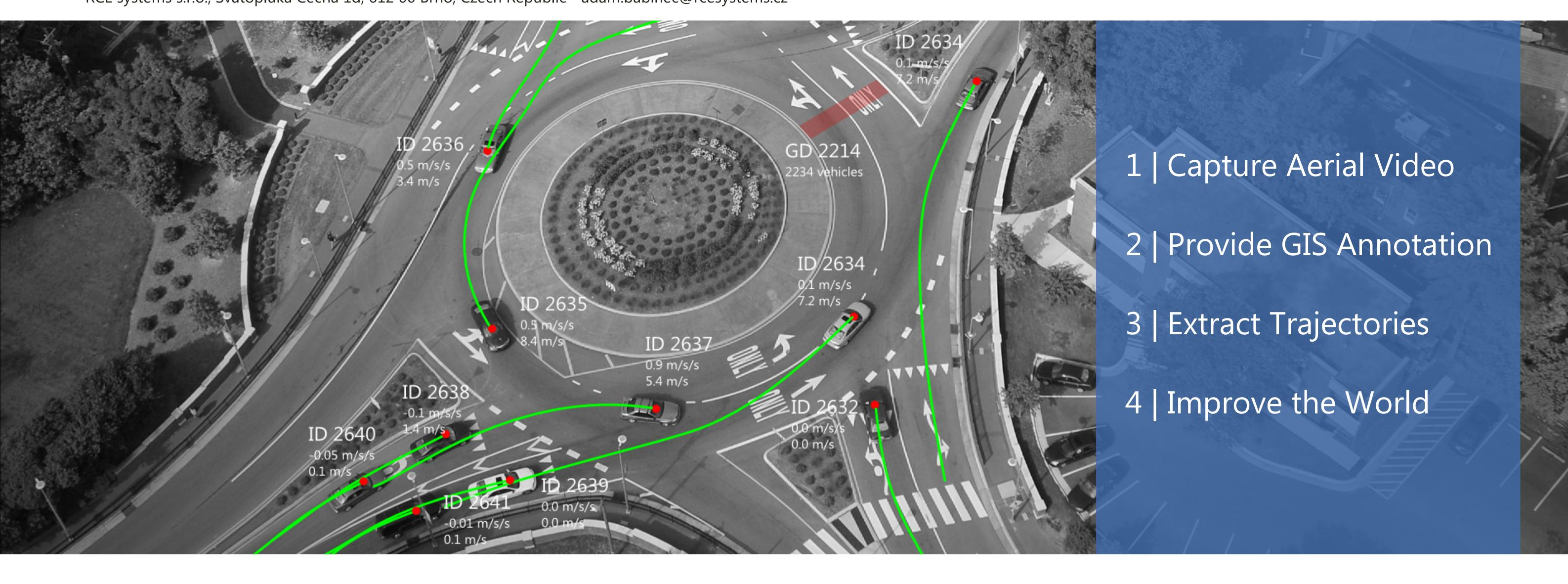
This poster presents a system for automatic vehicle trajectory extraction from aerial video data. The input video sequence can be captured by regular action camera mounted on a multicopter drone or balloon flying in altitudes from 40 to 200 m.
