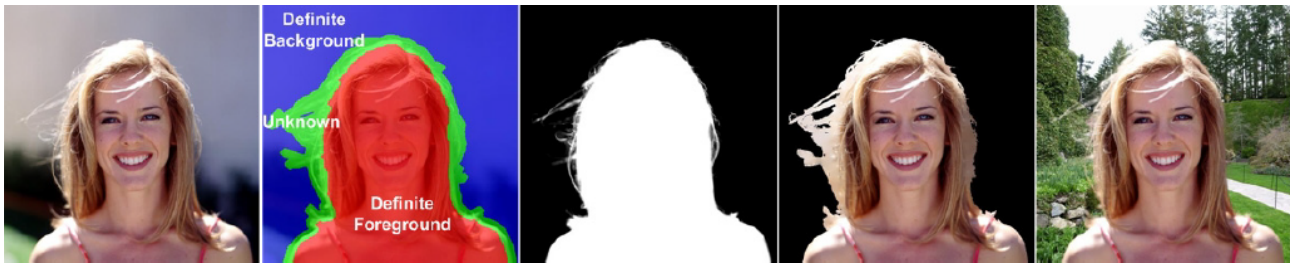
Figure 3. Example of the matting problem. From the left first : input image. Second: user-defined trimap (blue for background, red for foreground and green as an unknown region). Third: computed alpha mask. Fourth: original image without background (foreground area and unknown region are merged). Last: background is replaced. Figure is borrowed from book Image and Video Matting: A survey [7].
