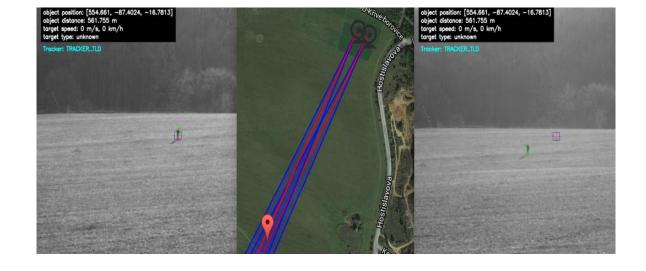
As for the static targets, nine landmarks with a priori known UTM coordinates (obtained from the cadastral map) and one target carrying an ordinary mobile GPS sensor were chosen. The system was tested against one dynamic terrestrial target equipped with a mobile GPS sensor (a walking person) as well. The target was tracked for 120 s and the estimated positions were captured and compared to the ground truth path; on average the system achieved the precision of 6.25 m.
