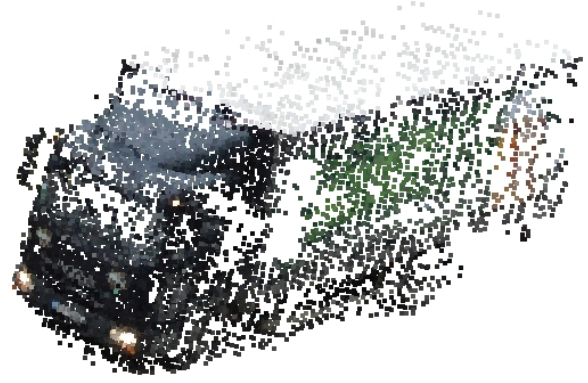
Figure 9. Resultant 3D reconstruction of a passing truck obtained when proposed improvements to Structure from Motion pipeline are applied.
