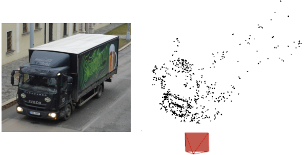
Figure 6. The best obtained result using COLMAP Structure from Motion tool for image sequence of passing vehicle. Resultant point cloud (on the right) contains recognizable front part of the truck.
