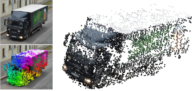
Figure 1. An example of keypoints found by modified correspondence search stage of 3D reconstruction pipeline (left) and the corresponding result of 3D reconstruction of a passing truck (right).
