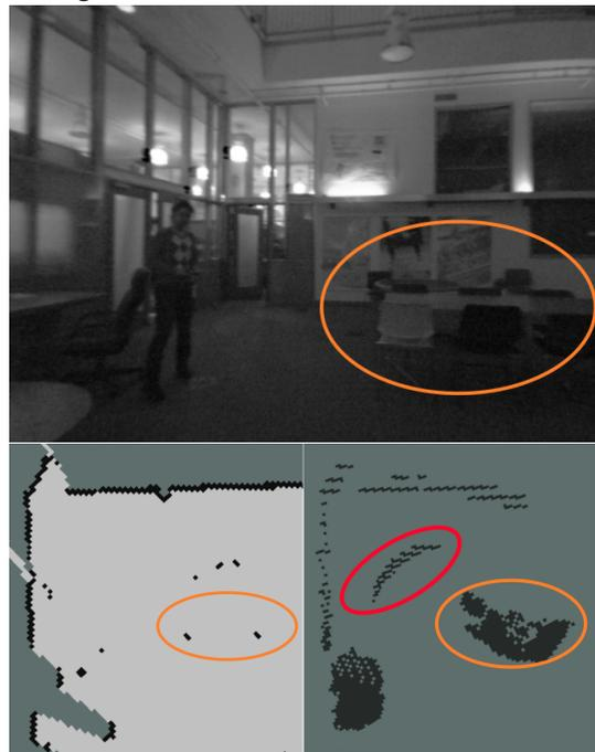
**Figure 11.** Table scene - source image on the top, LIDAR map at the bottom left, camera map at the bottom right.
