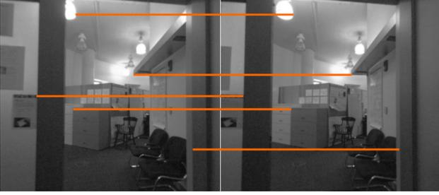
**Figure 2.** Pixel correspondences in left and right rectified images.
