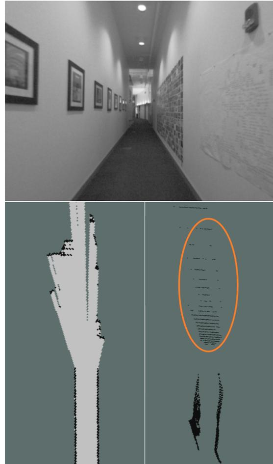
**Figure 10.** Passage scene - source image on the top, LIDAR map at the bottom left, camera map at the bottom right.
