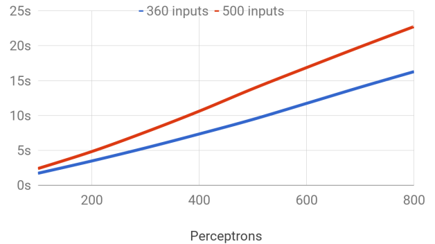
Figure 7. Comparison of the time required to process a single layer of a neural network in relation to the size of the layer. The number of perceptrons in a layer is shown on the bottom axis, layers with 360 inputs are drawn by a blue color, whereas the ones with 500 inputs are drawn by a red color.
