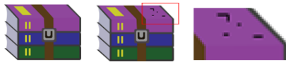
Figure 2. Icon modified with noise to evade classification based on exact match of cryptographic icon hash
