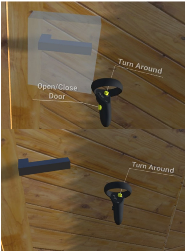
Figure 5. Upper image shows visualisation of ray-cast hitting door handle and the image below when the ray-cast is not hitting the handle.
