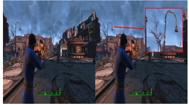
Figure 4. Visible visual artifact along edges in output of vorpX , when used for VR, suggesting use of steep parallax mapping for view duplication.
