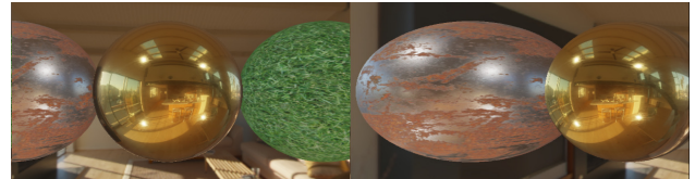
Figure 8. The same reflection on golden sphere's surface in side view (right) as in the front view (left), caused by missing propagation of altered transformation matrix to computation of camera-space position and pixel's normal in Fragment Shader.
