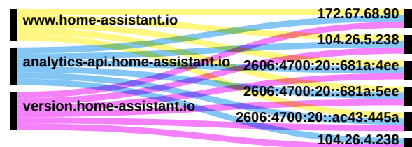
Figure 4. Diagram showing the running of multiple services on one endpoint—all three domain names under the *.home-assistant.io wildcard domain share the same IP address. Non overlapped relations are dismissed.
