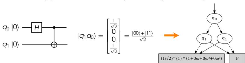
Figure 3: Circuit to create the Bell and its resulting MTBDD (leaf value F denotes zero probability amplitude)
