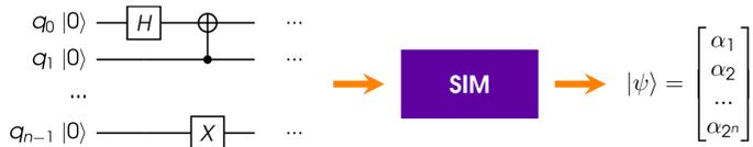
Figure 1: The aim of quantum simulation is to calculate the final state vector of the system
