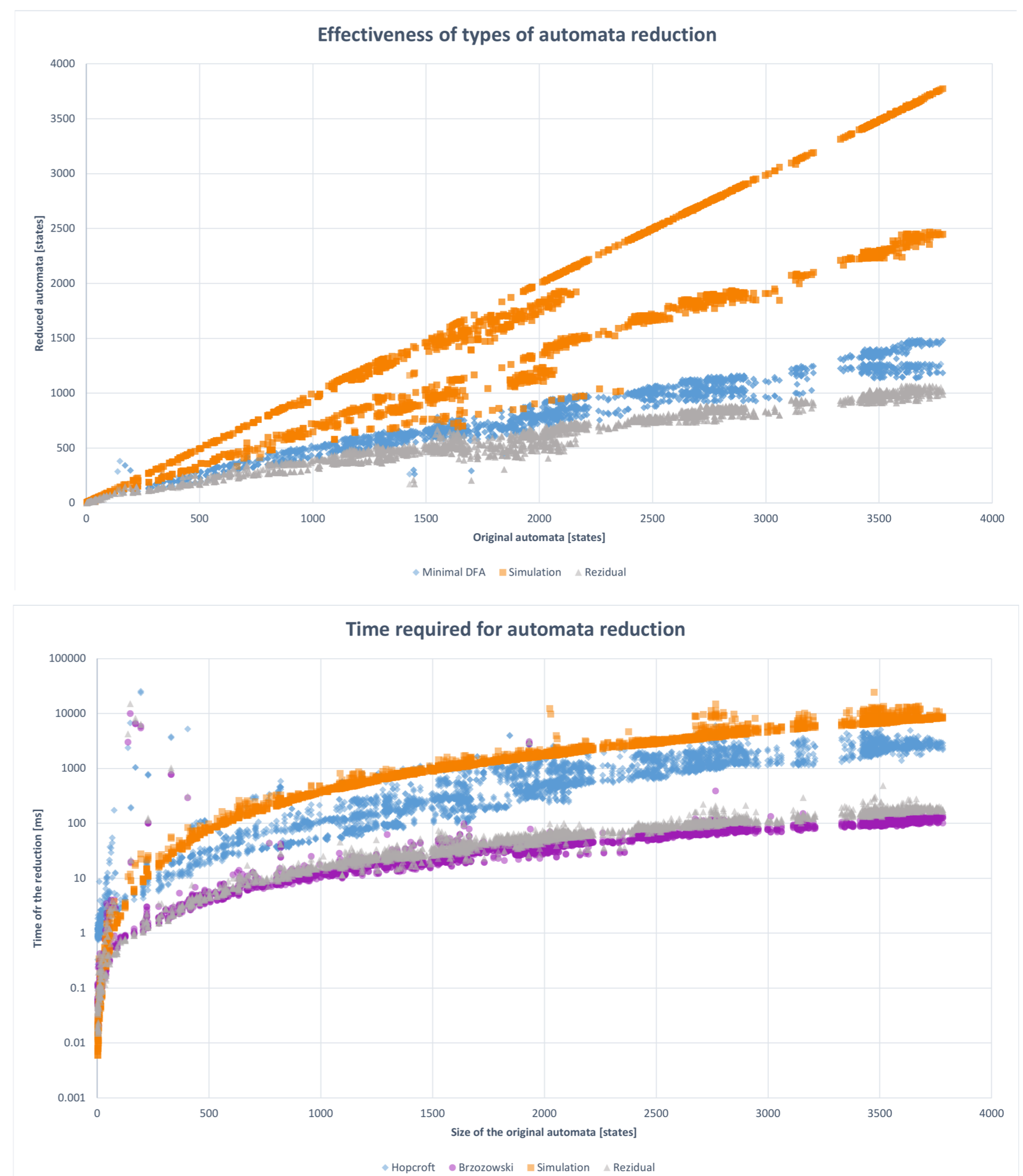
Figure 2: Graphs showing the results of implemented reduction algorithms, which are the minimization of DFA (using Hopcroft's and Brzozowski's algorithms), the reduction based on a relation of simulation, and the reduction utilizing residual automata.
